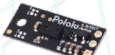
Proximity Sensor - Check if an artefact has reached the first shooting position and decide whether to sort or not
